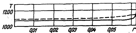
Fig. 1. Radial temperature profile of a reactor tube: obtained analytically (solid curve) and in an electrolytic trough (dashed curve).
